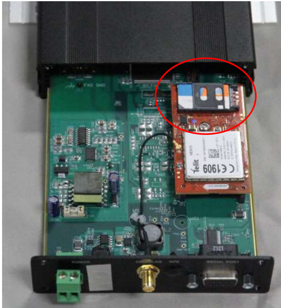
Figure 7. SIM card installed and locked into the SIM card holder.
