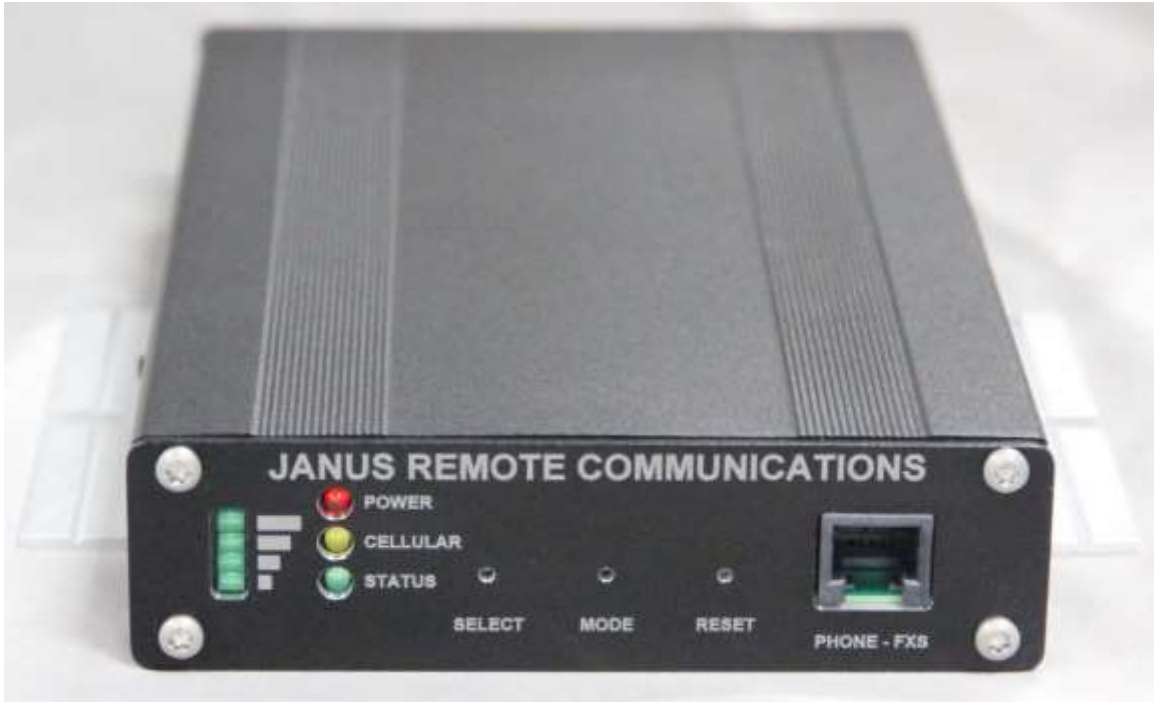
Figure 2. Front panel of the ETP-GSM Cellular Interface.
