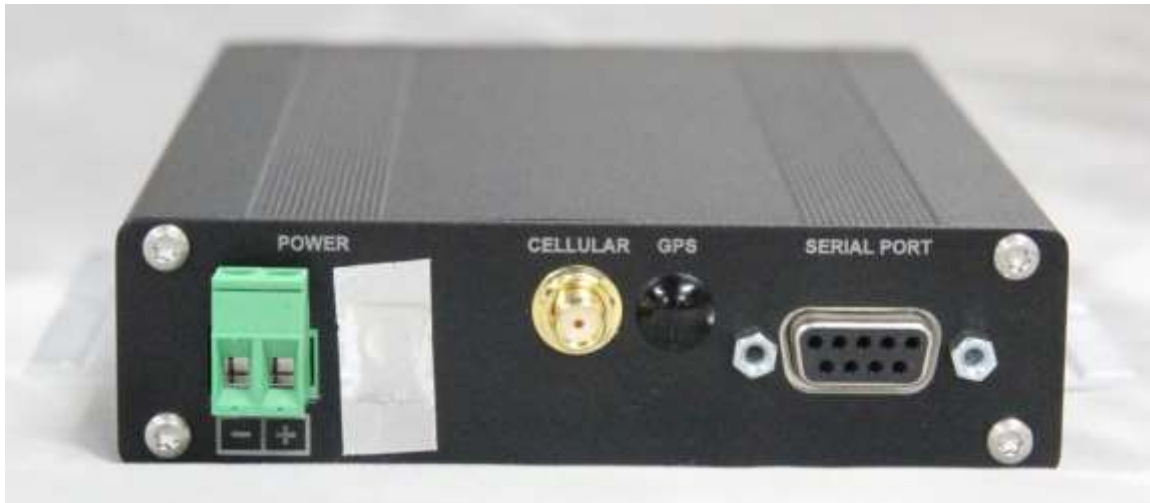
Figure 3. Rear panel of the ETP-GSM Cellular Interface.
