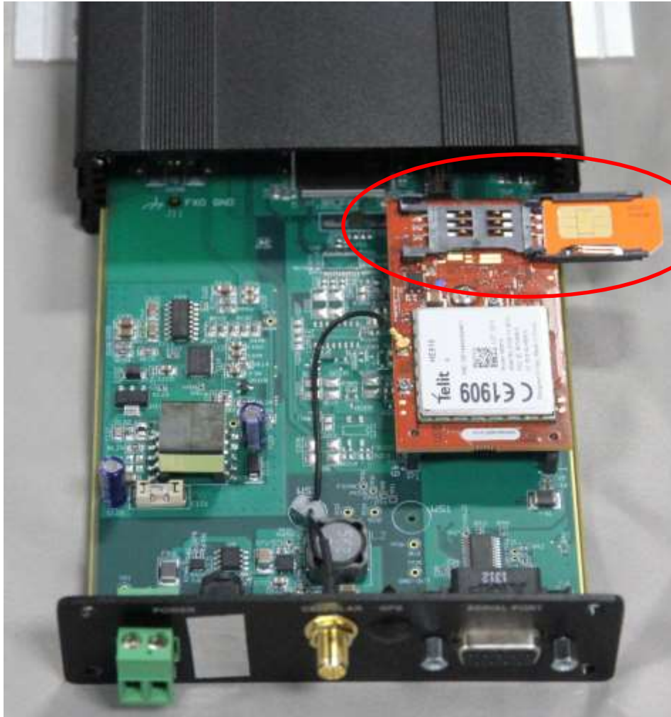
Figure 6. The tray of the SIM card holder in the open position. Note the SIM card that has been installed into the tray.
