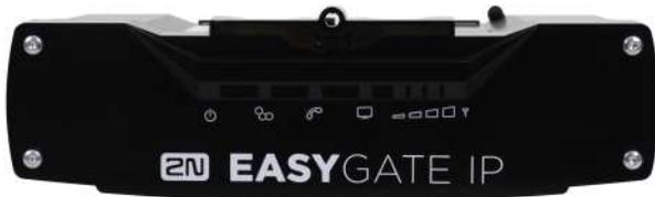
**2N® EasyGate IP** is designed primarily for voice transmission over VoIP (or VoLTE, GSM, UMTS) between a mobile network and a connected FXO-equipped terminal (PBX, phone, lift communicator, answering machine, etc.). When connected to the 2N® Elevator center cloud service, the gateway shows an extended functionality including remote management, auto provisioning, real-time device state monitoring and others.
