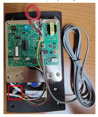
3. The ETP-120 Series includes one (1) Auxiliary Input and is optionally available in a configuration that provides one (1) Auxiliary Output (only model numbers with the **X** designator such as **ETP-120EX**).
