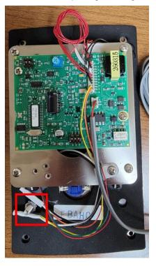
The AOR Series Analog Station includes one (1) Auxiliary Input and is optionally available in a configuration that provides one (1) Auxiliary Output (only model numbers with the -1RO designator). The optional single Auxiliary Output is rated at a maximum of 500 mA at 200VDC.
